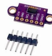
(e) O principal sensor do Lidar, o ToF VL53L0X
