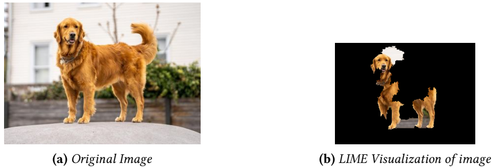
Figure 2.4: Visualization of top 15 most important superpixels for "Golden Retriever" ImageNet (RUSSAKOVSKY et al. , 2015) Class in image
