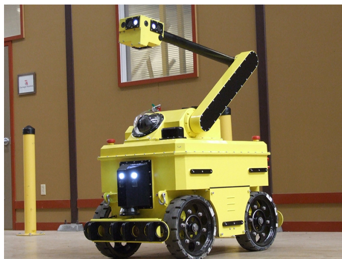
Figura 1 – Sensabot Inspection Robot
